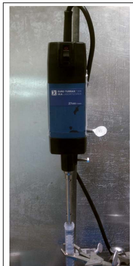
Figure 1. Homogenizer for generating nanoparticles.
