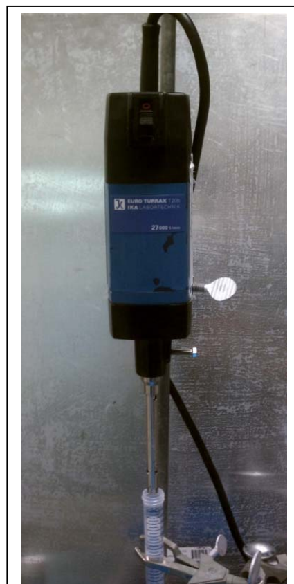
Figure 1. Homogenizer for generating nanoparticles.
