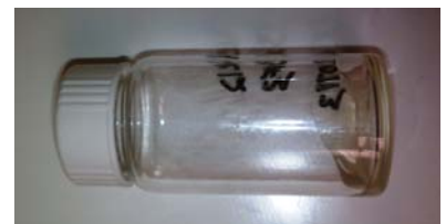
Figure 1. Vial containing ~1g PolyVivo AK12 in dry state. Appears like a semi-viscous gel.
